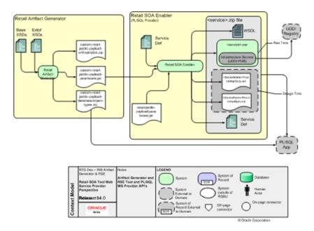
PL/SQL Applications (such as the Oracle Retail Merchandising System) use Oracle Objects, which are similar to the Oracle Retail RIB style APIs. The tool generates a Web service provider layer between the external clients and the PL/SQL APIs to provide the Web service functionality.
