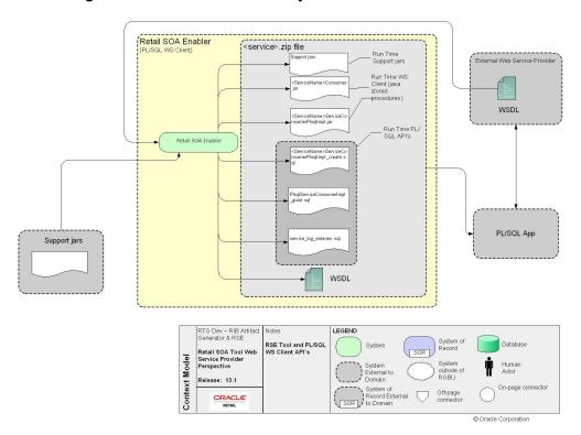
RSE tool requires a web service WSDL and the corresponding RSE's Service Def xml file as input for generating PLSQL service consumer code. The output of RSE is a zip file which contains all the artifacts required for invoking that WebService from PLSQL code. The output zip file follows the naming convention as <WebServiceName>PortType\_PlsqlWithJaxWsServiceConsumer.zip.
